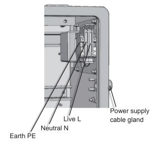
Fig. 4-25: Power supply connections
